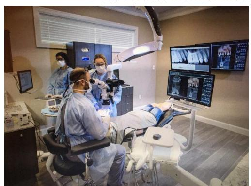
The dual vertical monitor mount, as shown, is for a dental chair. ICW's engineering team worked closely with the customer to create a special custom bracket and monitor mount to hold the monitors vertically with a tray and handle.
