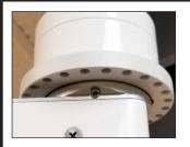
Rotation limits for the arm are set by placing stop pins in the holes where you want the arm to stop. The stop pins can be removed and set by hand.
