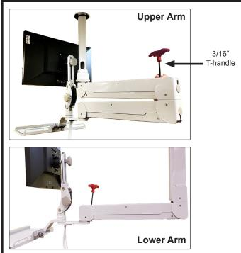
Extend the upper arm straight out as shown before adjusting the arm's lifting capacity. Be sure all equipment is mounted on the arm before adjusting. Adjust the arm closest to the monitor first. Use the 3/16" T-handle provided.
