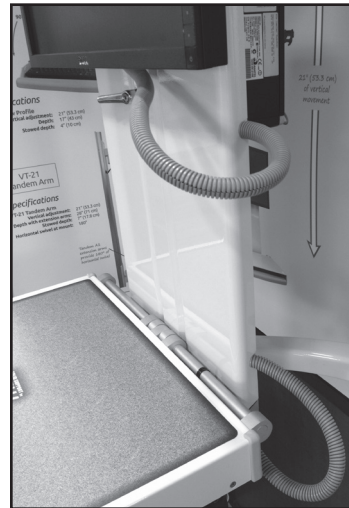
Wire management showing split wire loom.
