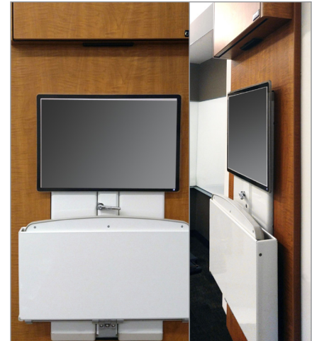
VT21 Low Profile mounted into a cabinet. Shown in the stowed position. Stowed depth 4" (10 cm), extended depth 17" (43 cm). The WorkSurface Tray provides a generous surface area for tasks. The VT21 series is available in three models: VT21, VTLP and VTTM.
