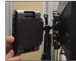
CPU with VQC plate shown being detached from back of monitor.
