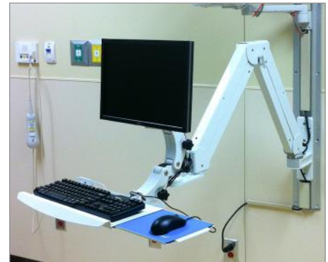
This mount attaches paralinks to both the monitor and keyboard, providing optional adjustment at four joints.
