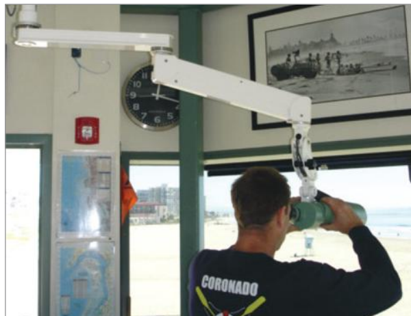
Shown above, a lifeguard tower telescope attaches to a paralink for additional freedom of movement.
