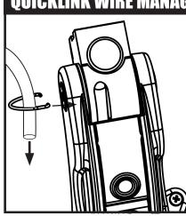
NOTE: The two clips provided can be installed on either side as needed.
