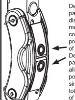
Depressing either paddle as shown will disengage the locking mechanism for the corresponding pivot providing 90 degrees of adjustment. Depressing both paddles as shown allows the user to position both pivots simultaneously for a total of 180 degrees of adjustment.
